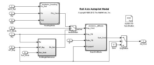
This model represents a basic roll axis autopilot with two operating modes: roll attitude hold and heading hold. The mode logic for these modes is external to this model. The model architecture represents the heading hold mode and basic roll attitude function as referenced models. The model includes:
